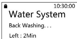
If you want to end up this step, press ESC key again. And the valve would go to the next working state immediately( if not, the valve can complete the regenerate progress itself). The rest working states of a regenerate progress are below:
